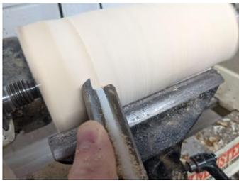
The Spindle Roughing Gouge
